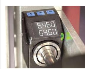
The SIKO position indicator AP05 with green status LEDs shows a correct machine setting. (Photo © SOMIC)
