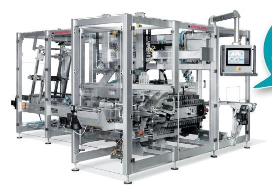
The ETIL end-of-line packaging machine for trays with lids enables a precise and product-friendly packaging process. Electronic SIKO position indicators for monitored size changeover can be integrated as an option.
