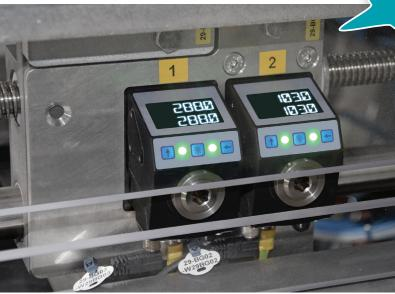
reliable as possible. Here, Rovema relies on SIKO's AP10 electronic position indicators with IO link interface for monitored and reliable size changeover, both for cartoning machines and for form-fill-seal machines.
