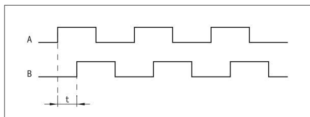
**Example: Pulse interval  $t = 1 \mu\text{s}$**
