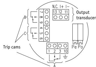
Fig. 6: Pin connection GP63/64 with Instrument transformer
