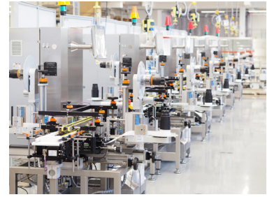
TQS serial numbering system with classical mechanical position indicators from SIKO (Image © WIPOTEC-OCS)
