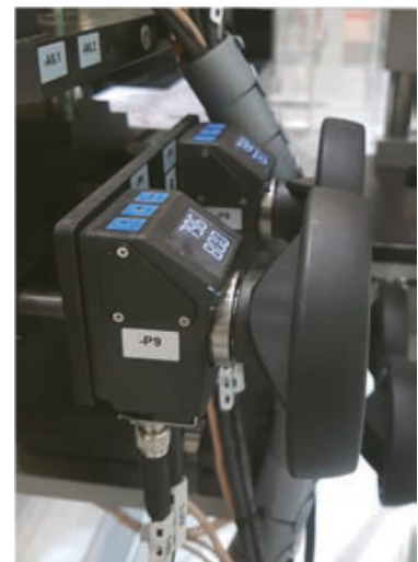
Bus-compatible electronic position indicator AP05 from SIKO that ensures secure and efficient transition to different folding box sizes (Image: © SIKO GmbH, Christian Fischer)
