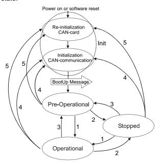
Fig. 1: CAN status diagram
