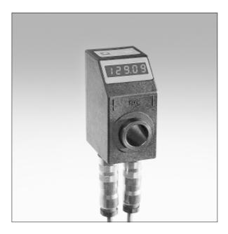
Absolute Electronic Indicator AP09 is used for applications requiring automatic data transmission of machine parameters via interface to a PC or control. Position and target values are indicated in the easily read LED-display. Easy mounting via hollow shaft plus the battery-backedup display allow a fast and safe machine set up.
