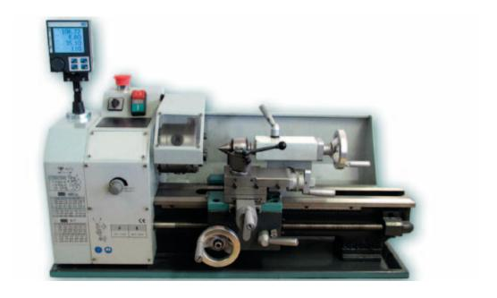
Accurate digital indication of the position values of the X, Y axes and simultaneous display of rotational speed. The illuminated display offers optimum readability under all conditions and provides the user with customizable display parameters.
